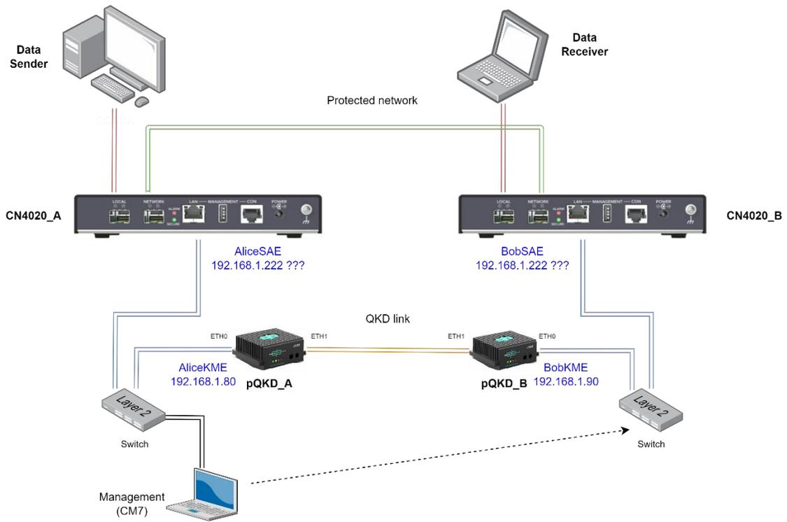
Figure 3 Network connection of CN4020s and pQKD devices
